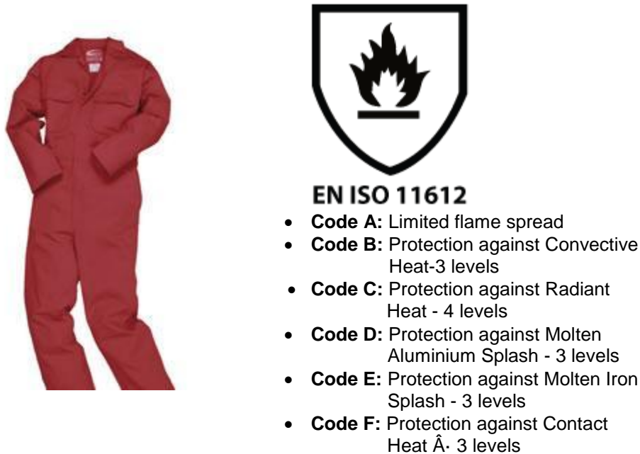
Figure 23: Indicative protective overall against heat and flame ISO 11612:2015 (source web)
